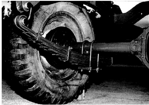
Figure 17.2 Leaf spring in an automobile.
